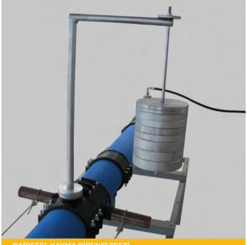
RESISTANCE TO PRESSURE DURING APPLICATION OF A BENDING MOMENT (M= 0,4D) TO THE BRANCH OUTLET
