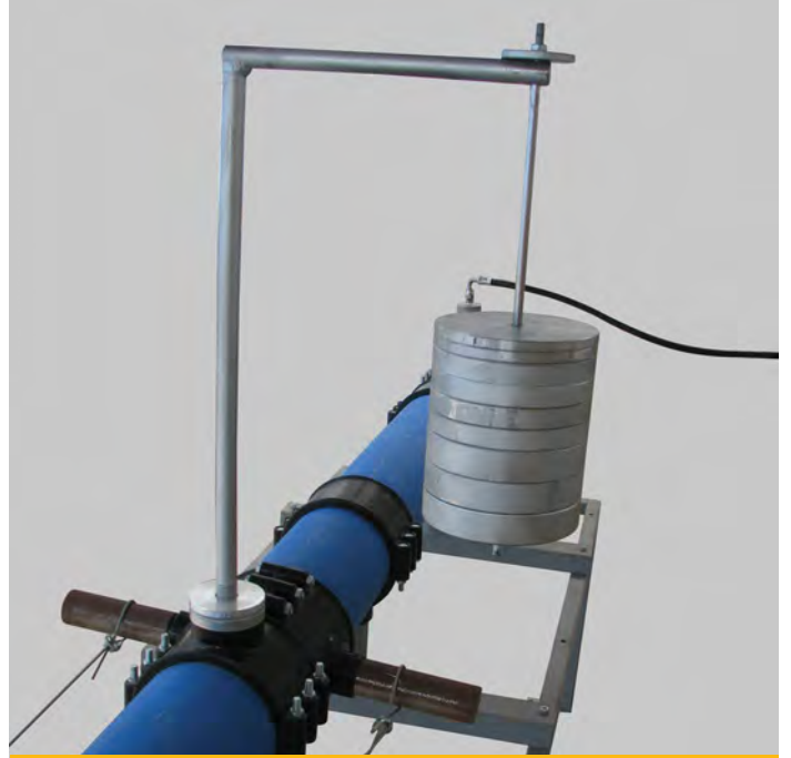
DAİRESEL KAYMA DİRENCİ TESTİ CIRCULAR SLIP RESISTANCE TEST
